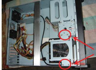
5. Safely route the AC power cord around the PSU and slide the entire unit into the slot
