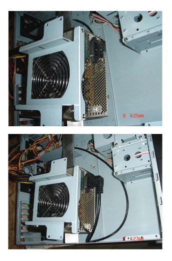
3. The Bracket should be securely tighten to the PSU
